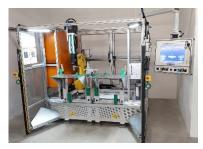
Image 1: TOX PRESSOTECHNIK developed a complete system for V-ZUG for the clinching of dishwasher housings.
