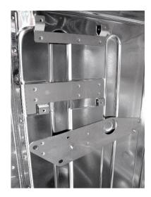
Image 6: The joining pattern of the TOX-Clinching points is clean and exact – an important criterion for the Swiss premium manufacturer.
